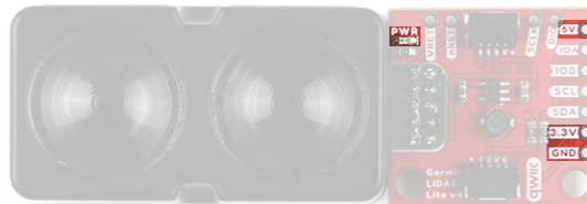
Power LED and power breakout pins on the Qwiic LIDAR-Lite v4. (Click to enlarge)
