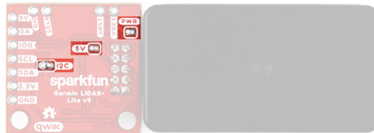
The power LED, I 2 C pull-up resistor, and 5V disconnect jumpers on the Qwiic LIDAR-Lite v4. (Click to enlarge)
