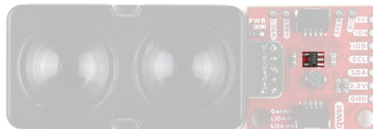
Boost converter on the Qwiic LIDAR-Lite v4. (Click to enlarge)
