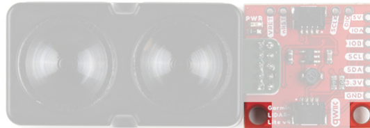
Screw holes and zip-tie notches on the Qwiic LIDAR-Lite v4. (Click to enlarge)
