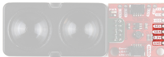
I 2 C Connections- The pins are tied to the Qwiic connectors.
