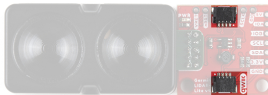
Qwiic connectors on the Qwiic LIDAR-Lite v4. (Click to enlarge)
