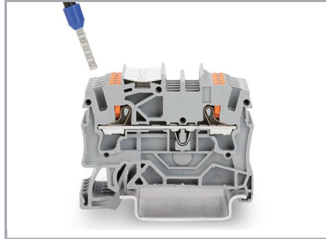
Push-in termination of solid and ferruled conductors
