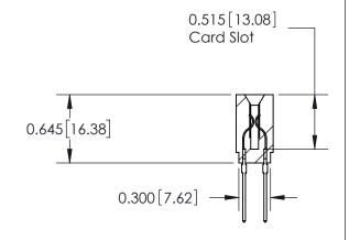
737 Series Ultra-Mate Card Edge Connector - Press Fit Part Number: 737-032-540-201 **EDAC INC** THESE DRAWINGS AND SPECIFICATIONS
