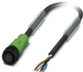
Sensor/Actuator cable, 4-position, PUR halogen-free, Black-gray RAL 7021, Free cable end, on Socket straight M12, A-coded, Cable length: 10 m, with plastic knurl
