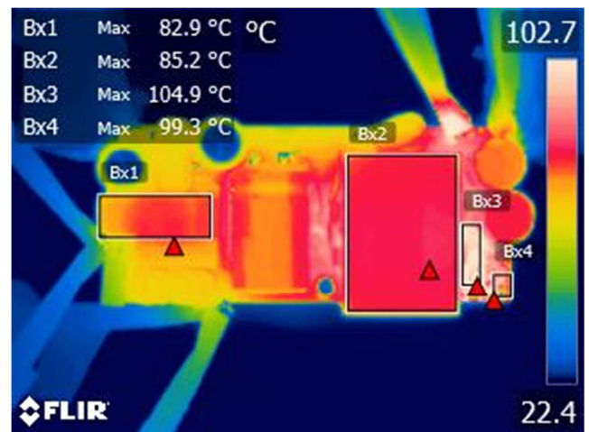
Figure 15 – Top Thermal Image, T_{AMB} = 22.4 °C. Bx1: Bridge, BR1 = 82.9 °C. Bx2: Transformer Core, T1 = 85.2 °C. Bx3: Secondary Winding, FL2/3 = 104.9 °C. Bx4: Snubber Resistor, R11 = 99.3 °C.
