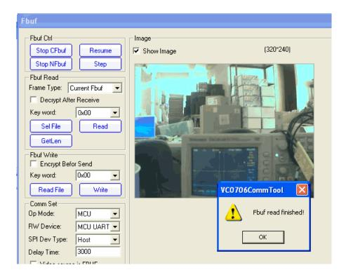
Thats it! You can now easily test reading camera images. To take another photo. Press **Resume** up at the top to have the video start up again. Then click **Stop CFbuf** when you want to snap another photo. Finally you can select the **Compression Ratio** which will improve or degrade the image quality but also change the image transfer time. There's no way to change the image size from this program (easily) but we can do it using the Arduino sketch so just try it out here to start.
