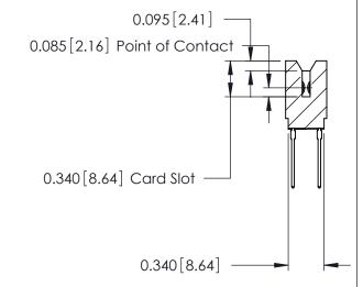
ACAD REFERENCE NO. 746 Series Ultra-Mate Card Edge Connector - Press Fit DRAWN: Part Number: 746-064-540-606 **EDAC INC** THESE DRAWINGS AND SPECIFICATIONS ARE THE PROPERTY OF EDAC INC.,AND TORONTO, ONTARIO SHALL NOT BE REPRODUCED, OR COPIED CANADA OR USED AS THE BASIS FOR THE MANUFACTURE OR SALE OF APPARATUS YOUR CONNECTION TO QUALITY & SERVICE WITHOUT WRITTEN PERMISSION.
