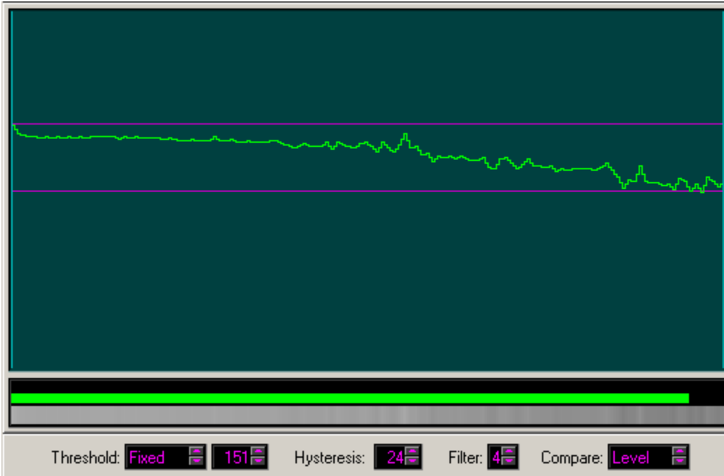
Intensity plot resulting from even illumination and a very slow readout.
