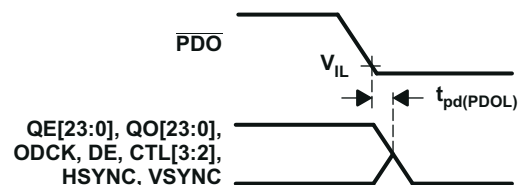
Figure 8-8. Delay From \overline{PDO} Low to Hi-Z Outputs
