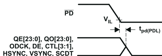
Figure 8-7. Delay From \overline{PD} Low to Hi-Z Outputs
