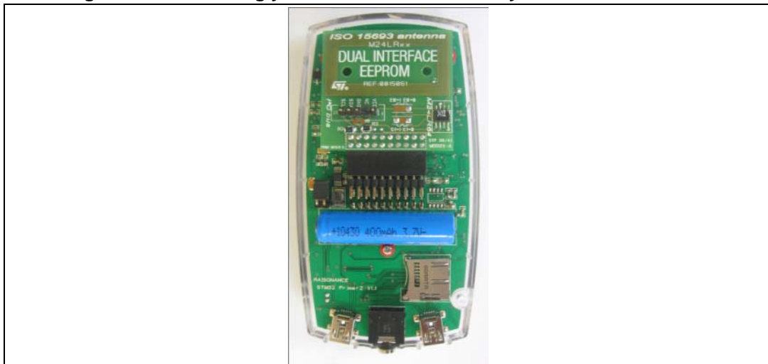
Figure 50. Connecting your reference antenna to your STM32-PRIMER2
