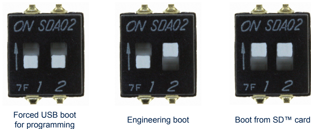
Figure 7. Boot-mode switch SW1
