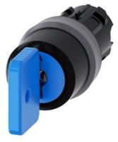
Key-operated switch O.M.R, 22 mm, round, plastic with metal front ring, lock number 73038, blue, with 2 keys, 3 switch positions I-O<II, left latching, right momentary contact type, actuating angle 2x45°, 10:30h/12h/13:30h, key removal O, with laser labeling, upper case and lower case, always upper case at beginning of line
