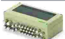
Item no.: 850-826 IP65 enclosure; Aluminium (RAL 7032); WxHxD (240x100x160 mm); 4 x M20, 4 x M16, 14 x M12 cable grip
