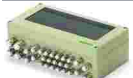
Item no.: 850-827 IP65 enclosure; Aluminium (RAL 7032); WxHxD (320x100x160 mm); 4 x M20, 8 x M16, 17 x M12 cable grip
