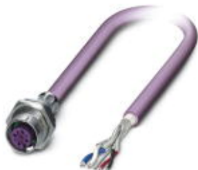
Bus system flush-type socket, DeviceNet/CANopen, 5-pos., M12, shielded, A-coded, Speedcon, rear/screw mounting with Pg9 thread, with 0.5 m bus cable, 2 x 0.2 mm 2 ; 2 x 0.32 mm 2
