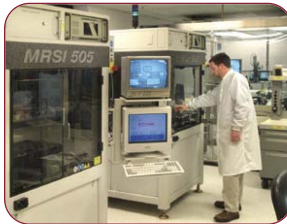
AUTOMATED EPOXY AND DIE PLACEMENT
