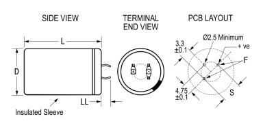
General Information Series ALC70 Dielectric Aluminum Electrolytic Description Snap-In, Aluminum Electrolytic RoHS Lead 3 Pin Short AEC-Q200 No Halogen Free Yes Component Weight 50 g Notes Dimensions D And L Include Sleeving. Shelf Life 156 Weeks
