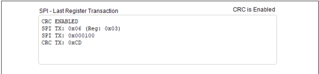
Figure 6. SPI Write Transaction with CRC Enabled
