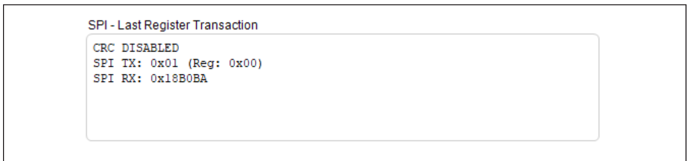
Figure 4. SPI Read Transaction with CRC Disabled
