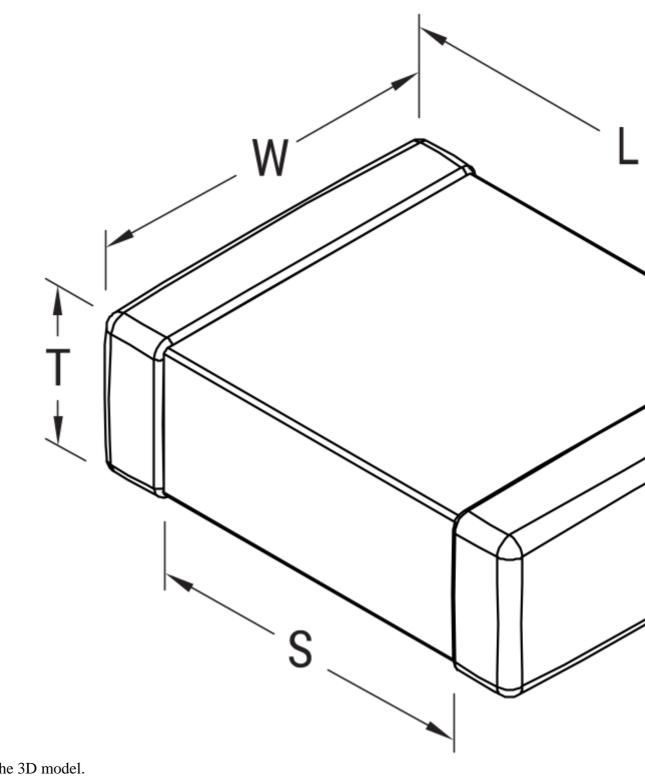
Click <u>here</u> for the 3D model. Dimensions Chip Size 0402 L 1mm +/-0.05mm
