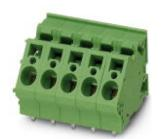
PCB terminal block, nominal current: 32 A, pitch: 7.5 mm, number of positions: 4, connection method: Spring-cage connection, mounting: Wave soldering, conductor/PCB connection direction: 45 °, color: multi-color
