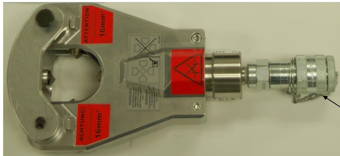
CT-980CH DIE-LESS, FLIP-TOP CRIMP HEAD TOOL
