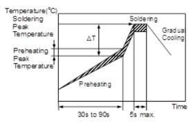
[Standard Conditions for Flow Soldering]
