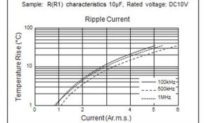
[Example of Temperature Rise (Heat Generation) in Chip
