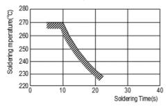
In the case of repeated soldering, the accumulated soldering time must be within the range shown above.
