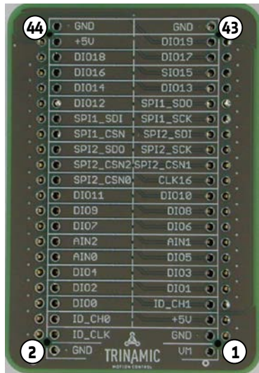
Figure 3.3 Eselsbrücke: pin assignment
