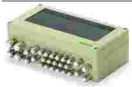
Item no.: 850-827 IP65 enclosure; Aluminium (RAL 7032); WxHxD (320x100x160 mm); 4 x M20, 8 x M16, 17 x M12 cable grip
