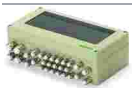
Item no.: 850-828 IP65 enclosure; Aluminium (RAL 7032); WxHxD (480x100x160 mm); 4 x M20, 10 x M16, 35 x M12 cable grip
