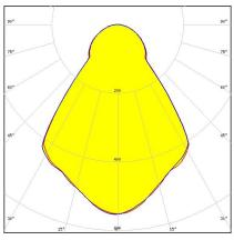
Dimensions: 16.1 mm x 16.1 mm Height: 10.10 mm Mini reflector with ~60° wide beam and clip installation
