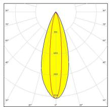
Dimensions: 16.0 mm x 16.0 mm Height: 9.50 mm ~35° + 15° oval beam. Assembly with holder and installation tape. Pin position
