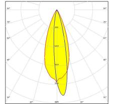
Dimensions: 16.1 mm x 16.1 mm Height: 9.70 mm Asymmetric beam for wall-washing.
