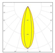
**Dimensions: 16.1 mm x 16.1 mm Height: 11.00 mm** ~35° + 15° oval beam optimized for Nichia NS6x83. Assembly with holder and installation tape.
