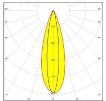
**Dimensions: 16.0 mm x 16.0 mm Height: 9.50 mm** ~35° + 15° oval beam. Assembly with holder, installation tape and location pins.
