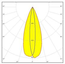
Dimensions: 16.1 mm x 16.1 mm Height: 9.70 mm ~35° + 15° oval beam. Assembly with
