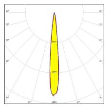
Dimensions: 16.1 mm x 16.1 mm Height: 9.70 mm ~14° spot beam. Assembly with holder and installation tape.
