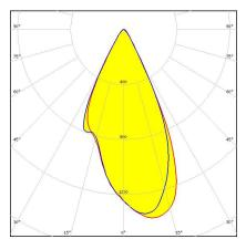
Dimensions: 16.1 mm x 16.1 mm Height: 9.70 mm ~45° wide beam. Assembly with holder and installation tape.
