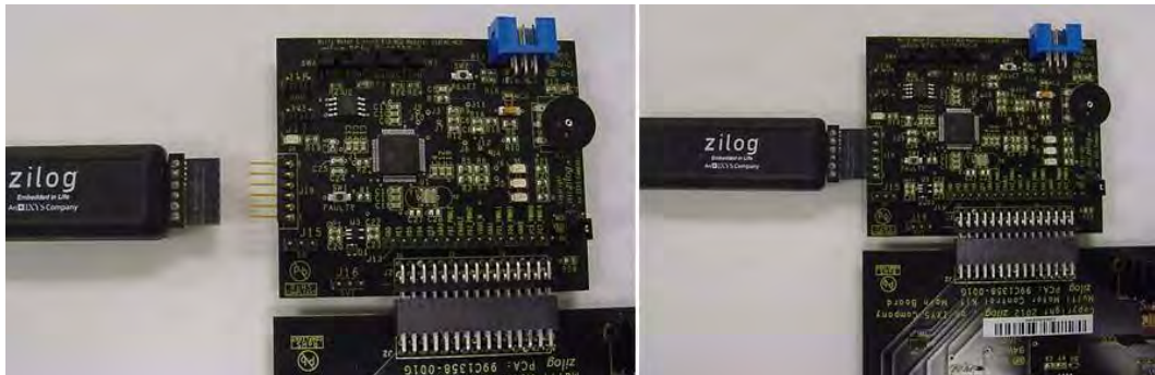
Figure 5. The Opto-Isolated USB Connection to the UART Adapter
