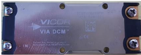
Previous chassis mount terminal hardware (Philips head)
