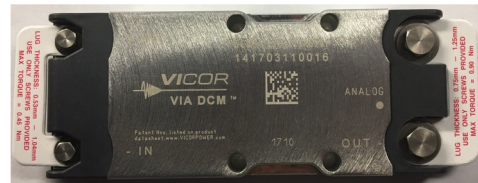
Revised chassis mount terminal hardware Input: M3 x 0.5, 4 mm hex head Output: M3.5 x 0.6, 6 mm hex head
