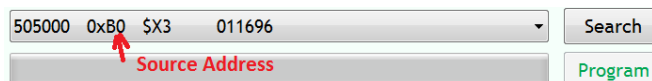
Figure 20: The location of desired controller's source address in the Main Menu Window.
