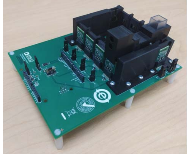
Figure 9. Fully Assembled EVAL-CN0503-ARDZ Setup
