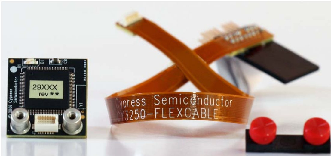
Figure 3-3. Flex Cable and 29000-28 DIP
