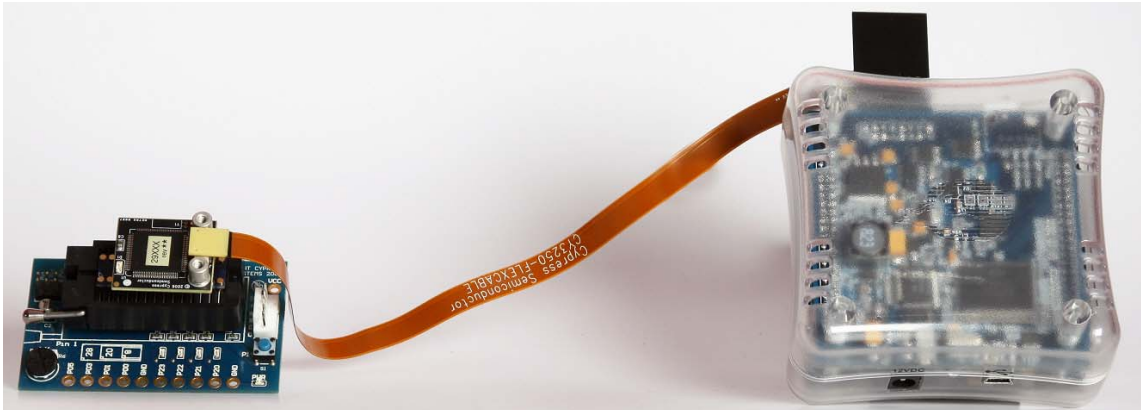
Figure 3-7. Flex Pod Connected to ICE-Cube Pod
