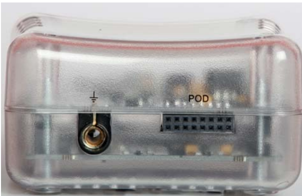
Figure 3-9. Connector in ICE-Cube
