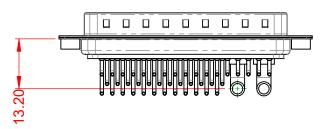
40A (CURRENT) POWER/CO-AX CONTACT RATING: (IF PRESENT) SIGNAL CONTACT CURRENT RATING: 5A PER CONTACT SIGNAL CONTACT RESISTANCE:  $10m\Omega$  MAX. INSULATOR RESISTANCE: 5000MΩ min.
