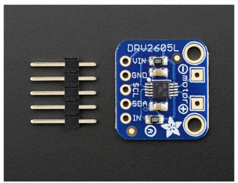
This chip is controlled over I2C - after initialization, a 'string' of multiple effects can be strung together in
