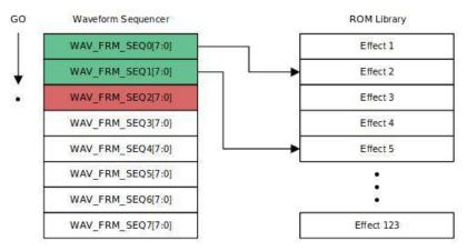
You access the Waveform Sequencer by using the **sequence** property and providing an index for the slot location. To specify the effect, use the special **Effect** class provided in the library, giving it the effect
