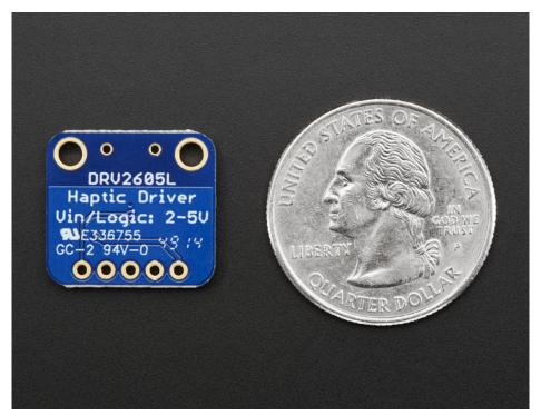
According to the product page, it can be used with both LRA (Linear Resonance Actuator) and ERM (Eccentric Rotating Mass) type motors but we have only used it with our little vibration pancake ERM. (https://adafru.it/dDc)
