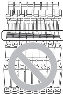
Incorrect installation Some terminals not inserted completely.
