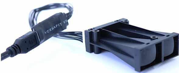
Figure 6: TOF>range 611 and USB-UART adapter
