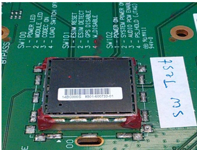
Figure 10. Glue deposit on WP module.
