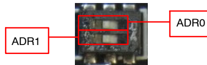
Figure 6. Address Switch Locations in their Default Positions. The First Switch (ADR0) and the Second Switch (ADR1) of SW3 are Set to ON
