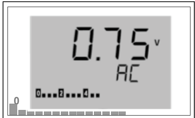
Figure 9. AC voltage display
