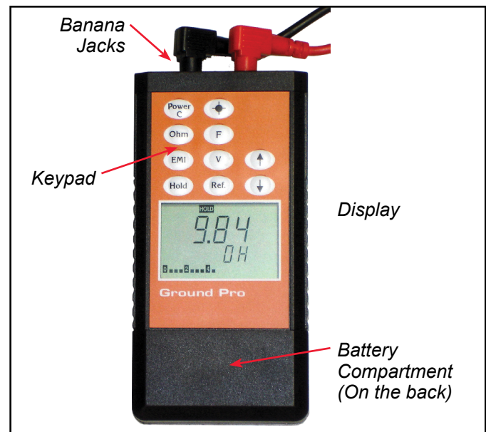
Figure 2. Ground Pro Meter features and components
