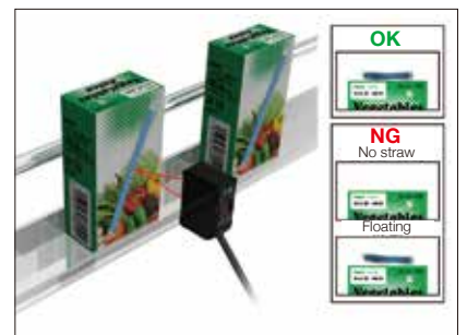
Detecting straws and float (Output 1: ON with no straw; Output 2: ON when floating)
