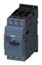
Circuit breaker size S2 for transformer protection A-release 9.5...14 A N-release 328 A screw terminal Standard switching capacity
