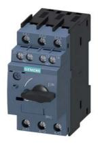
Circuit breaker size S00 for transformer protection A-release 7...10 A N-release 208 A screw terminal Standard switching capacity with transverse auxiliary switches 1 NO+1 NC
