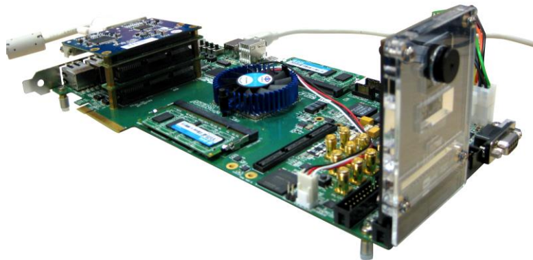
Figure 3-1 The Connection Setup for DE4 users
