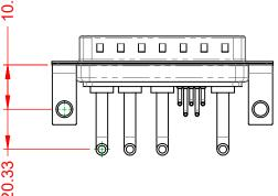
POWER/CO-AX CONTACT RATING: (IF PRESENT) SIGNAL CONTACT CURRENT RATING: 5A PER CONTACT SIGNAL CONTACT RESISTANCE:  $10m\Omega$  MAX.
