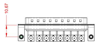
75Ω (IMPEDANCE) **POWER/CO-AX CONTACT RATING:** (IF PRESENT) SIGNAL CONTACT CURRENT RATING: 5A PER CONTACT SIGNAL CONTACT RESISTANCE:  $10m\Omega$  MAX. **INSULATOR RESISTANCE:** 5000MΩ min. DIELECTRIC
