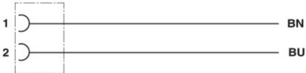
Contact assignment of 7/8" socket
