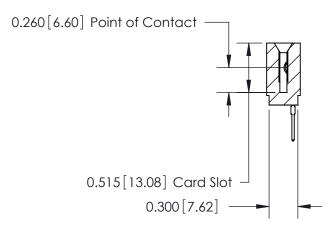
745 Series Ultra-Mate Card Edge Connector - Press Fit Part Number: 745-052-522-101 **EDAC INC** THESE DRAWINGS AND SPECIFICATIONS
