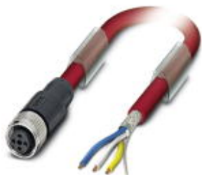
Bus system cable, CC link (10 Mbps), 4-position, PVC, red, shielded, free cable end, on Socket straight M12, A-coded, cable length: 5 m
