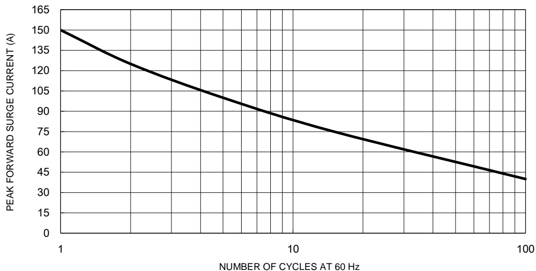
Fig.5 Maximum Non-Repetitive Forward Surge Current
