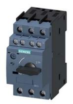
Circuit breaker size S0 for motor protection, CLASS 10 A-release 4.5...6.3 A N-release 82 A screw terminal Standard switching capacity with transverse auxiliary switches 1 NO+1 NC
