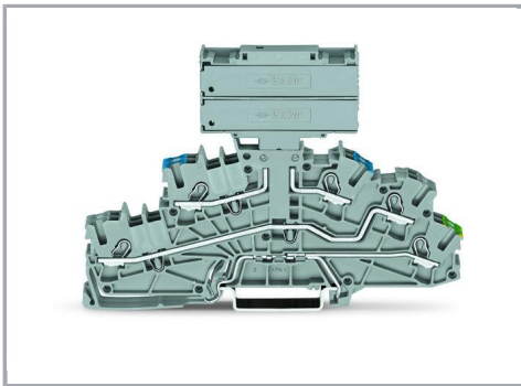
Double-fuse plugs with (5 x 20) mm glass cartridge fuses can be used on carrier terminal blocks without an N-knife disconnect in standard terminal block width.
