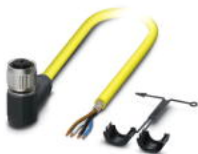
Sensor/actuator cable, 4-position, PVC, yellow, shielded, free cable end, on Socket angled M12 SPEEDCON, A-coded, cable length: 10 m
