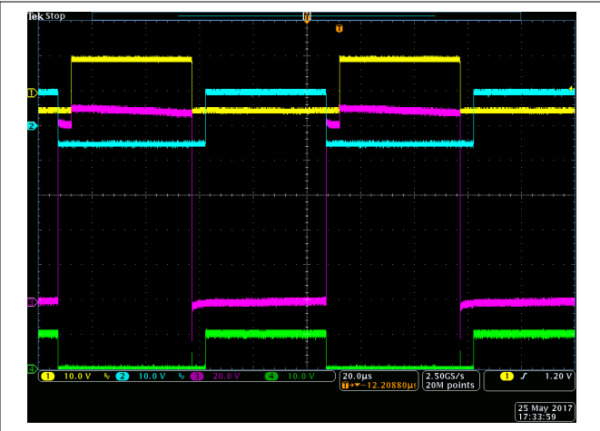
Figure 8-10. Input Negative Voltage
